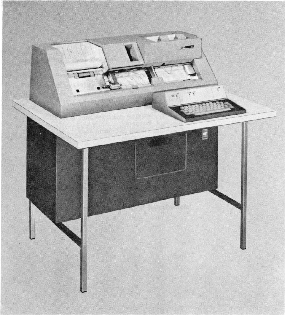
Figure 1-1. IBM 29 Card Punch, with Left-Zero Insertion
